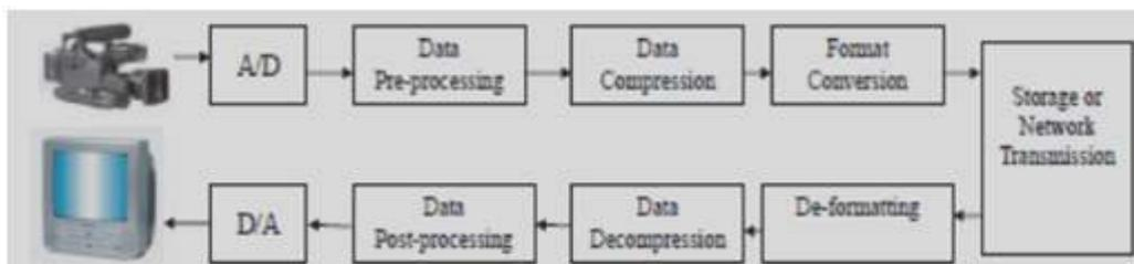
Figure 1: an Example of a digital video system
