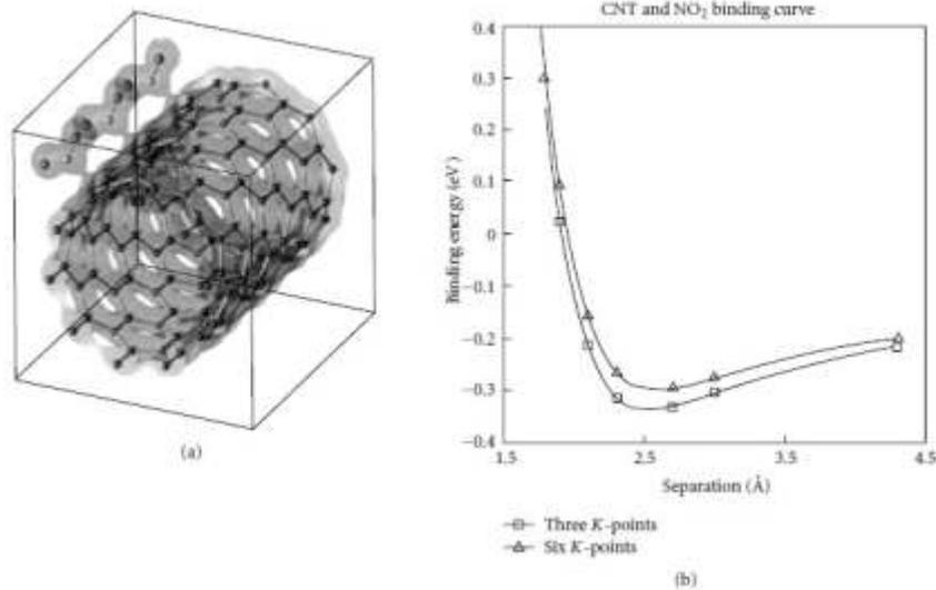
Fig 1: (a) Total valence electron charge density plot. The value of charge contour is 0.0015 (e/Å<sup>3</sup>) showing the binding charge between the SWNT and the NO<sub>2</sub> molecule. Three units are shown in this figure.
