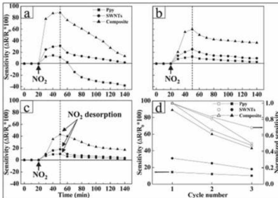
**Fig. 2:** The change of sensitivity as a function of gas exposure time at an NO<sub>2</sub> concentration of 3000ppm: (a) Annealed Sample (b) the second cycle after 24hr (c) the third cycle after 48 hr. (d) the change in sensitivity as a function of cycle no. [16]
